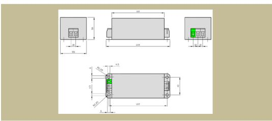
It is intended for military and special purposes and also where higher attenuation is necessary. When connecting it is necessary to meet the EMC requirements for its proper function, i. e. as short PE connection as possible and to avoid paralleling of inlet and outlet from the filter.
