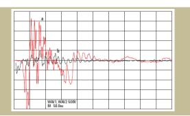
The diagram illustrates the reduction of rapid voltage pulses (switching overvoltage), which are led into the input of the extension cord.
