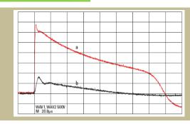
The diagram illustrates the amplitude reduction of impulse wave leading into the input of extension cord. Shape of impulse wave according to standard ČSN EN 61000-4-5 (a) had amplitude 3,5 kV. The amplitude of the impulse wave at the receptacle outlets was 800 V (b). Time axis of the diagram is 20  $\mu s$  / piece.
