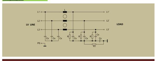
It is used to frequency converters and appliances which need supplemental interference suppression. For example: soft starters, pulse resources, thyristor controls, electronic units and whole switchboards.
