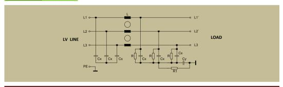
It is used to frequency converters and appliances which need supplemental interference suppression. For example: soft starters, pulse resources, thyristor controls, electronic units and whole switchboards.
